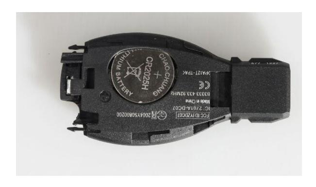
4. Push the metal strips on both sides into the right position.
