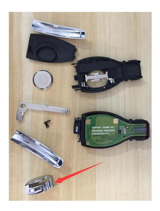
Note: If the rear metal component is firstly assembled, then the metal strips on both sides won't be able to put into the right position.
